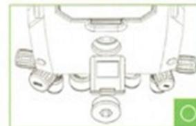
4. Tighten the filter replacement bolt using a hexagon wrench.
